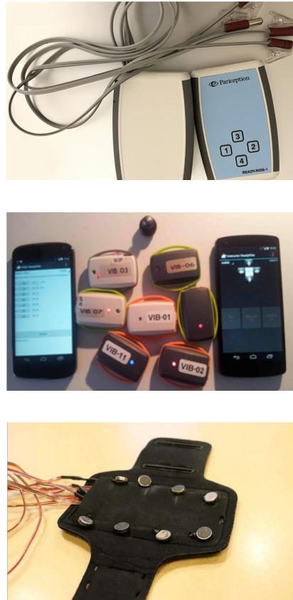
Figure 16: Pictures of the devices Ready-Ride, Ready-Move and Vibro-Braille (from top to bottom).
